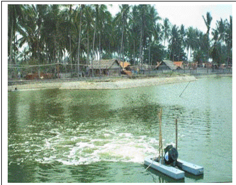
FIGURE 6.2. Typical pond application of a propeller-driven, electrically powered air aspiration system. (Source: Aeration Industries International Inc., Minneapolis, MN.)
